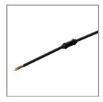
Ordering Code: 0532-0-9-000-00 Cable H07RN-F 3x1sqmm length 500mm. with anti-humidity kit.[pre-assembled from factory]
