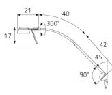
An easily located reading luminaire for hospital environments with plastic-coated sprung arm for easy cleaning.
